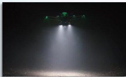
应急照明 Emergency lighting
